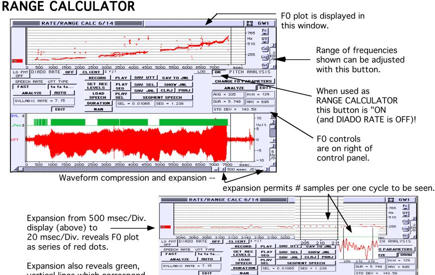
vertical lines which correspond to peaks in the F0 plot. — SoundScope uses these to determine vibratory cycles. "Holes" in plot can be edited or eliminated.
